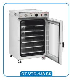
Vacuum Tray Dryer used in various industries under vacuum atmosphere to dry temperature-sensitive materials. It gives complete drying and vaporization of moisture of the product. Inside Chamber made of S.S. (304) & Outer Mild steel duly powder coated / S.S. Temperature controlled by Microprocessor based PID Controller, Temp. Stability ±1°C, Temperature Range 50°C to 130°C. It Fitted with Vacuum Release Valve, with Toughened Glass Door, Provided with S.S. Trav. Tray size 16" x 32".
