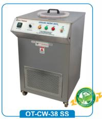
Double-walled Inner Chamber S.S. 304 & Outer M.S. Duly Powder Coated / S.S. 304. PUF Insulated Temp. Range 5°C to 50°C Cooling Compressor. Copper Cooling Coils Welded throughout on the Outside of the S.S. Chamber. Body Mounted on sturdy Angle Iron Frame with Caster wheels for easy movability. Temperature controlled by Microprocessor Based PID Controller, provided with circulating Pump.
