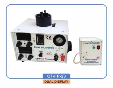
A solution of the salt is aspirated into the LPG-AIR flame. The vapour takes up energy from the flame and emits the wavelength characteristic colour of the element being tested. The intensity of emitted light is proportional to the concentration of the metal ion in the solution.
