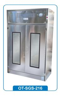
These specially designed cabinets provide a wash of sterile filtered, clean air through Imported Mini Pleat HEPA Filters having an efficiency of 99.97% down to 0.3 micron particle size. This cabinet protects dust and other particulates on clean room garments or other materials. For use in the change Room for garment storage & inside the clean room for storage of materials. Self standing cabinet provides down flow clean air to clean room garments.
