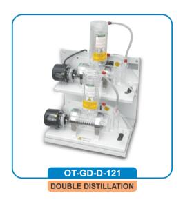
The distillation apparatus consists of boiler with heating elements embedded in glass and fused in spiral type coil internally of the bottom and tapered round glass, suitable to work on 220 Volts 50 Cycles AC complete with metallic stand rings and clamps to hold boiler condenser electric board with switch and connecting cords. It is capable of producing pure distilled water. Also the whole unit can be hanged on wall.
