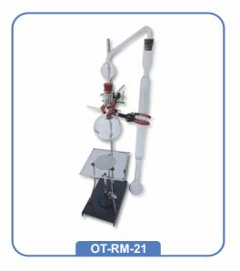
R M Value Apparatus, also known as Polenske's Apparatus is fabricated from Borosilicate Glass and used for determining butterfat, soluble and insoluble volatile acids in fats and oils. It comprises of 300ml flask still head, condenser and receiver flask graduated at 100 and 110 ml.
