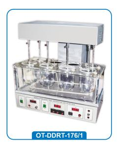
The Apparatus is same as the above but for six stages. The unit is equipped with, acrylic water bath controlled by digital temperature controller which is normally set at 37°C and duly fitted with pump which recirculates the water thus maintaining homogeneous temperature. The acrylic water bath is with digital timer can be set ranging from 1 to 999 minutes add it "BEEPS" at the end of the set time.
