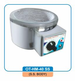
Most suitable for labs, pharmaceuticals, chemical glass plants etc. Useful for heating inflammable liquids electric heating net is hand knitted from glass yarn (without any joint) and for durability & stands. Temperature up to 350°C. The body is made of Mild Steel duly powder coated / S.S. 304. Mantles lagged with special grade mineral wool. Most suitable to work on 220 volts A.C. Supply.
