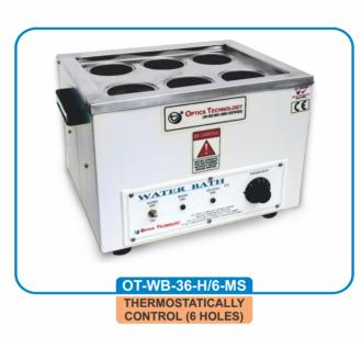
(Double walled) Inner chamber made of Stainless Steel 304 & outer made of S.S. 304 / Mild steel duly Powder Coated. The top has 75 mm holes with concentric rings. Temperature ranges upto 99°C. Accuracy  $\pm$ 5°C in thermostatically Controlled fitted with Neon Lamp indicator, main switch and workable on 220 Volt, 50 Hz. A.C.
