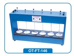
Fitted with D.C. MOTOR But to work on 220 Volts A.C. with Variable Speed from 20 R.P.M. to 100 R.P.M. approx. Jar Test Apparatus allows efficient and economical flocculation matter and collides in general and also has been specially designed for use in water treatments to correctly estimate the dosing of alum and such other coagulants for treatment of Water sewage and flocculation formation test in Water Treatment plants.
