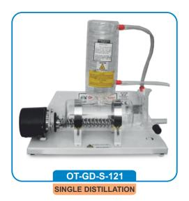
The distillation apparatus consists of boiler with heating elements embedded in glass and fused in spiral type coil internally of the bottom and tapered round glass, suitable to work on 220 Volts 50 Cycles AC complete with metallic stand rings and clamps to hold boiler condenser electric board with switch and connecting cords. It is capable of producing pure distilled water. Also the whole unit can be hanged on wall.
