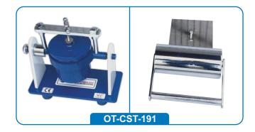
The test is used for determining liquid absorptiveness or resilience of treated and untreated paper, board, fabrics and other sheet materials. The test consists of a test apparatus, its 10kg roller and blotting paper. The roller method is recommended to insure better consistency and reliability that can be obtained by manual blotting or rubbing the specimen.
