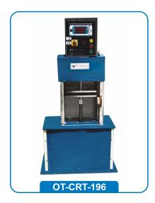
Crush Testers are designed for performing Ring Crush Test (RCT), Edge Crush Test (ECT), Flat Crush Test (FCT), Pin Adhesive Test (PAT), Concora Medium Test (CMT), Corrugated Crush Test (CCT) and other general compression tests, on a variety of materials like paper, paperboard etc.
