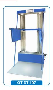
Drop tester manual / electrically operated auto model for determination of transport worthiness of packed containers.
