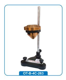
A simple significance device that permits the timed flow of a known level of liquid passing through an orifice located at the bottom. The conditions in a simple flow cup are rarely ideal for making true measurements of viscosity. It is important when using a Ford Cup and when retesting liquids that the temperature of the cup and the liquid is maintained, as ambient temperature makes a significant difference to viscosity and thus flow rate.
