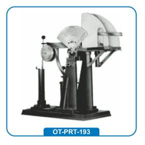
The puncture resistance Tester is used for determine the puncture of corrugated board by measuring of energy required to puncture it. Interchangeable weight supplied to cover four energy ranges i.e. in new meter 0-5, 0-10, 0-20 & 0-36.
