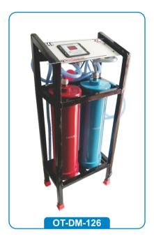
It consist of an inbuilt prefilter & very high exchanging capacity non-corrosive CATION & ANION Resin, columns prefilled with imported Resins for efficient results having treated water parameters. Fitted with a sturdy PVC multi control valve & can be connected direct to water taps. Fitted with analog / digital conductivity meter. Supplied with one plastic chemical proof regeneration tank & the complete unit is housed in a painted M.S. trolly for easy mobility.
