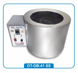
**Double walled** inside chamber are made of S.S 304 & outside made of M.S. duly powder coated / S.S 304 & gap between two walls is fitted with high grade glass wool to minimize thermal loss.
