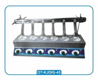
The digestion units are provided a condensing tap with individual condensing taps. They are placed on a MS angle stand with their respective controls supplied with/without any glass parts. Works on 220V mains Supply. It is used to determine organic nitrogen (N<sub>2</sub>) content in the substance.
