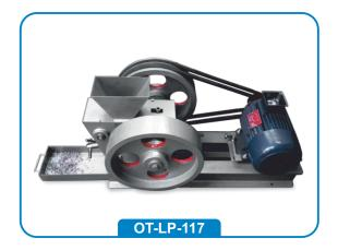
We are engaged in offering a very highly premium quality range of Laboratory Pulverizer. It is a self contained grinder, with a rotary disc, having a planetary movement in a vertical plane. Laboratory Pulverizer is a disc type grinder, designed to grind virtually any material to produce a fine mesh sample in one operation. It is a self contained grinder, with a rotary disc, having a planetary movement in a vertical plane.
