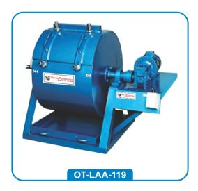
This machine is for determining the resistance to wear off small size coarse aggregates and crushed rock. The machine consists of a hollow cylinder, mounted on a sturdy frame on ball bearings. A detachable shelf which extends throughout the inside length of the drum catches the abrasive charge and does not allow it to fall on the cover. The drum is rotated by an electric motor through a heavy duty reduction gear.
