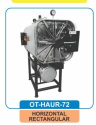
Inner chamber jacket and boiler is made of stainless steel. Sterilization cycle is controlled by three way valve or multi port valve. It is fitted with automatic pressure control switch, (indfoss piezostat), safety valve, pressure gauge, pressure release valve, water level indicator with cord & plug. Lid is made of S.S. 304 with water level cut-off device & Digital Temperature Controller Cum Timer.
