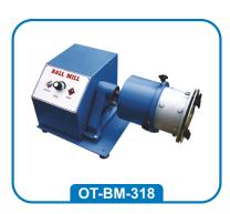
For mixing & grinding, electrically operated having capacity upto 2 Kg. Fitted with geared Motor with variable speed. The jar is made of S.S. and having steel balls of different sizes to be put in jar for mixing & grinding pesticides powder. Jar is available in aluminium and S.S.
