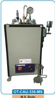
Cement Autoclave comes with great accuracy and is a cost-effective model for conductive accelerated soundness test of the cement.
