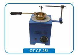
Cleveland Flash and Fire Point Appratus is determine of flash and fire points of petroleum and other liquids except Fuel oils and those materials having an open cup Flash 79°C to 400°C.
