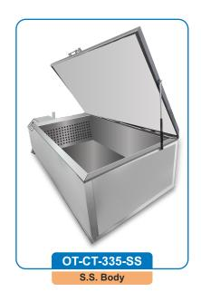
The tank has been designed to accommodate casted cubes and fully insulated, complete with a hinged lid, heater, thermostat and recirculation pump. Provision of two removable racks allowing free circulation of water around each cube.
