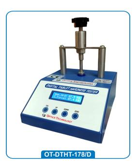
Tablet breaking force (commonly known as Tablet Hardness) is a measure of mechanical integrity of a tablet. It is widely used in pharmaceutical industries and research institutions.
