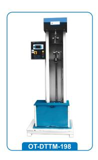
It is based on the Constant Rate of Traverse (CRT) principle. The sample is held between two jaws, the upper one is a stationary jaw while the other end is made to move at a known fixed speed with the help of Motor, Gear Box and Lead Screw arrangement. The load exerted on the Stationary jaw is sensed by a sensor connected with load cell which directly indicates the load in Digital form in Newton and kg.
