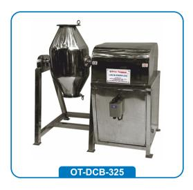
It is a type of mixer that can use to produce a homogenous solid mixer mainly use for material like semolina flour & pharmaceutical granules.
