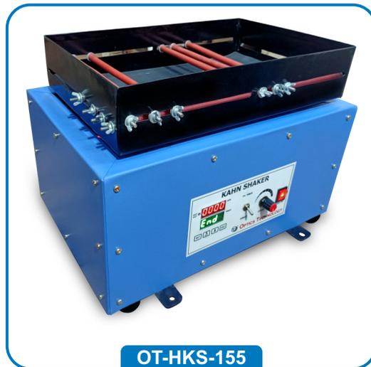
D.C. Motor special system shaker to work on 220 Volts A.C. for variable and smooth function speed control by speed regulator. It is general purpose machine and found useful for mixing or agitation ingredients, solution in flasks, bottles, beakers and kahn racks etc. Upper tray covered with rubber floor and sides of the tray are slotted to take parallel and cross bars cover with rubber. The bars are tightened with washers and fly nuts which can be adjusted as per the requirement.
