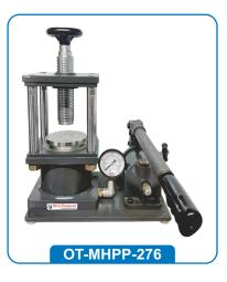
"**Optics Technology**" manually operated Hydraulic Pallet Press for fast and easy preparation of both solid and highly permeable pellet.
