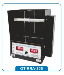
This instrument meant for determining neuro-pixicity, muscle tone, balance and motor co-ordination in rats and mice. A versatile built with LSI chips is equipped with Two compartments. Digital milliseconds timer for measuring the fall-off time of the mice.
