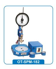
For testing penetration in grease/ creams. It consists of a vertical pillar mounted on a base, the head, together with diameter plunger rod and cone (or needle) slides on a pillar and can be clamped at any desired height. The dial graduate from 0 to 400 in 1/10 millimeter subdivisions. Supplied with a penetration needle, ring weights and two sample containers with Digital Timer.
