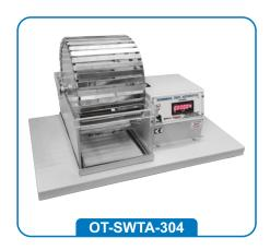
The locomotor activity can be easily measured using SWIMMING TEST APPARATUS which consists of clear perspex rotating drum with ribs in a clear perspex tank and Digital counter with resetting facility to count the activity of the animal. Both rats and mice may be used for testing in this apparatus. This Apparatus consists of ONE DRUM and perspex tank as described above for testing.
