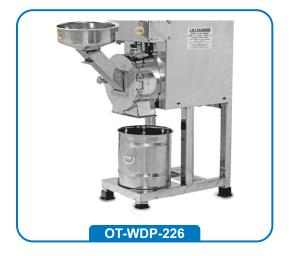
Made from heavy duty basically for large scale purpose. The product to be wet grinded are grounded in two / three stage operation depending on fineness desired.
