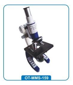
Monocular microscopes are often used in classrooms and laboratories for observing slide samples and it is an instrument for viewing small things through a single lens.
